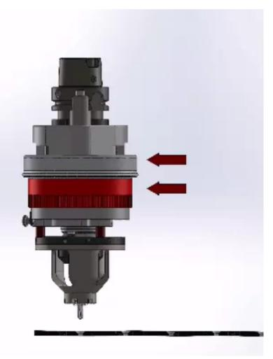
Compensation of the shape deviations through the use of a Floating Aggregate.
