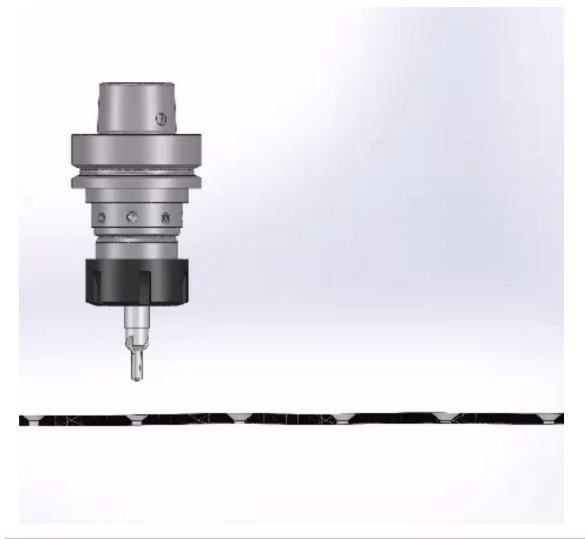
Different depths of the countersinks due to shape deviations of the material.
